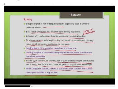
So, now let me summarize whatever we have discussed in this lecture 11. So, we know that the scraper is good at both loading, hauling and it can dump and spread the material in layers of uniform thickness. So, that is advantage that makes it more versatile, it is both good in loading and hauling and it can be used for depositing the material your dumping and spreading can be done in one continuous operation.
