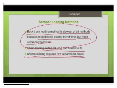
So, to summarize back-track loading method is the slowest of all the methods because of the additional pusher travel time for backtracking on returning. But most commonly followed because people prefer cutting in same direction. Chain loading, it is suited for long and a narrow cut, here
