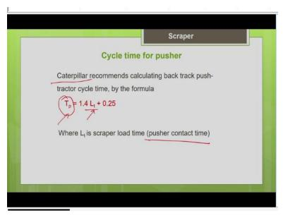
So, there is a thumb rule formula given by the caterpillar to determine the cycle time of the pusher, if you know the loading time of the scraper you can determine the cycle time of the pusher. Tp is the pusher cycle time and Lt is the scraper load time, the contact time of the pusher with your scraper during the loading phase of the scraper. So, if you know the loading time you can calculate the pusher time using this formula.
